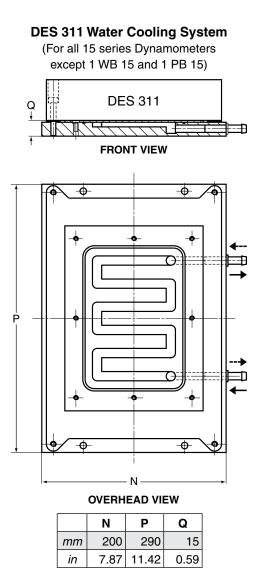
The DES 310/DES 311 supplies are delivered with integrated cables (including connectors) with a length of 1.5 meters on the dynamometer connection side and 5 meters on the controller side. The DES 310/DES 311 units are to be mounted on a metallic surface in order to allow ample heat dissipation. For 3–4 WB 15 and 4 PB 15 dynamometers, the DES311/131 Power Supply with integrated Water Cooling System (see above drawing) should be used.
